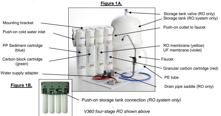
Keep in mind that you may install a tube tee on the line to the faucet to connect icemakers or other faucets to the system. If you locate your system farther than 20 feet from the faucet, you will need to add a pressure booster pump to your system. See your dealer for parts and details.
